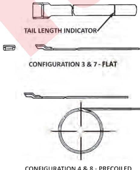
M85049/128-1, M85049/128-2, M85049/128-5, and M85049/128-6 Welded Buckle Bands
