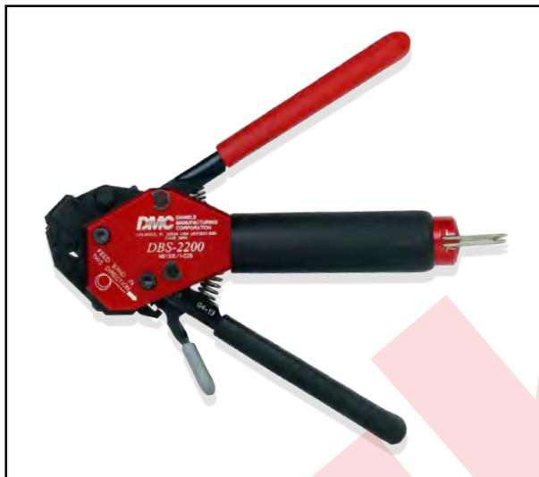
DMC's One-Step Banding Tools are designated for **M85049/128-3**, **M85049/128-4**, **M85049/128-7** and **M85049/128-8** "stamped buckle" bands. These tools tension, bend, and cut the band in one operation.
