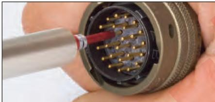
**Typical application showing tool testing pin contacts.**
