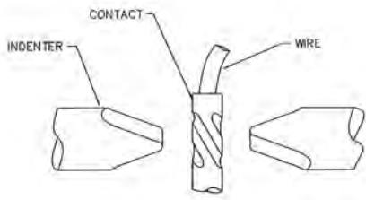
The model **SC8** has single flat-tipped indenters and accommodates wire sizes 12 thru 26 AWG (the miniature to sub-miniature range). It accommodates the TP series positioners and is easily identified by a distinctive black body and grey handle grip. It is 9 $\frac{1}{4}$ " in length and weighs approximately 15 oz. Gaging is accomplished with the G125 "GO/NO-GO" gage.
