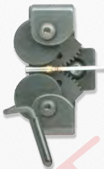
15-3202C Cam Grip Standard Contact Grip Terminal Lugs, Machined Contacts
